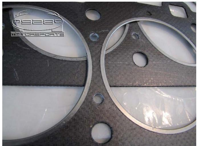
**Step 1:** Lay our head gaskets onto your heads and mark the center of each of the 6 vent holes per head gasket. You will see two of them near where the cylinders are closest to each other.
