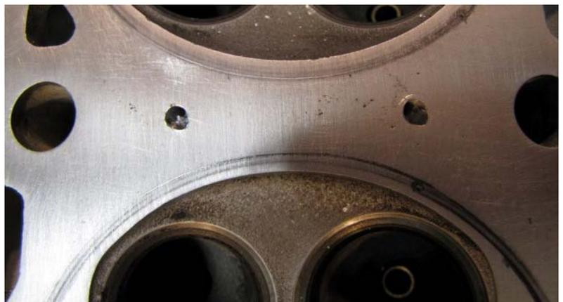
**Step 4:** Now change to a 7/32" drill bit and clean the top of each starter hole with it.
