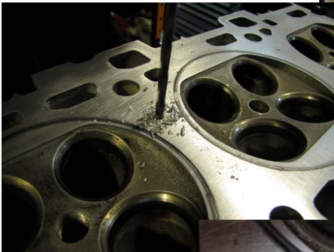
**Step 2:** With a 3/16" drill bit, drill down only 1/8" in each of the 6 marked vents per head. These are starter holes, and will combine the vents into a common entrance point.
