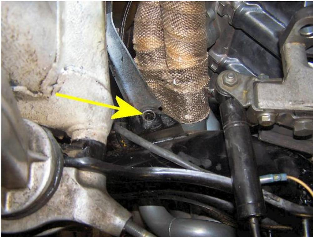
15. From under the car again, locate and remove the last two cross-member – to – frame bolts. They are at the extreme ends of the cross-member on the L and R sides, near the rear lower a-arm mount.
