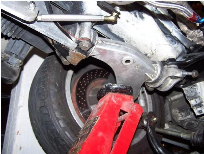
4. While the floor-jack is holding it up, start all the bolts in to the lower a-arms caps and the forward straps that you removed in steps 10,11,12 above. Use anti-seize compound on the threads. Spin them up into place, but do not fully tighten these bolts at this time.
