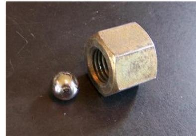
Be careful not to lose the metal ball inside the cap! Save the cap and ball in a bag for later in case you ever want to put them back on.
