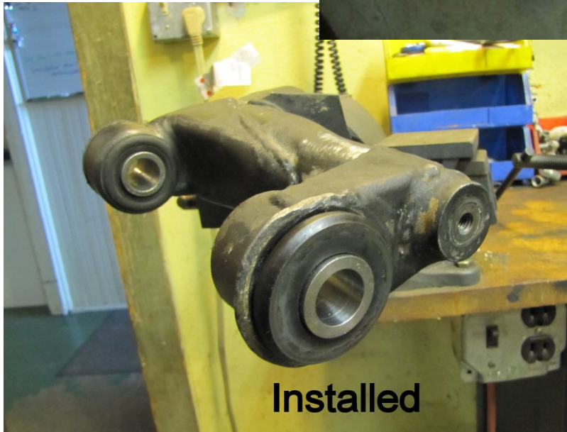
Finished new bushing installation.
