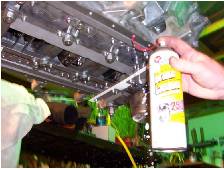
Clean the threaded holes with Brake Cleaner
