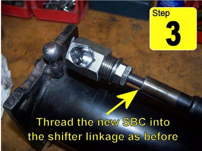
Threading the forward shifter rod on to the new ball cup is made easier if you pull the shift knob off, the shifter boot, and disconnect the forward shifter rod from the bottom of the shifter.
