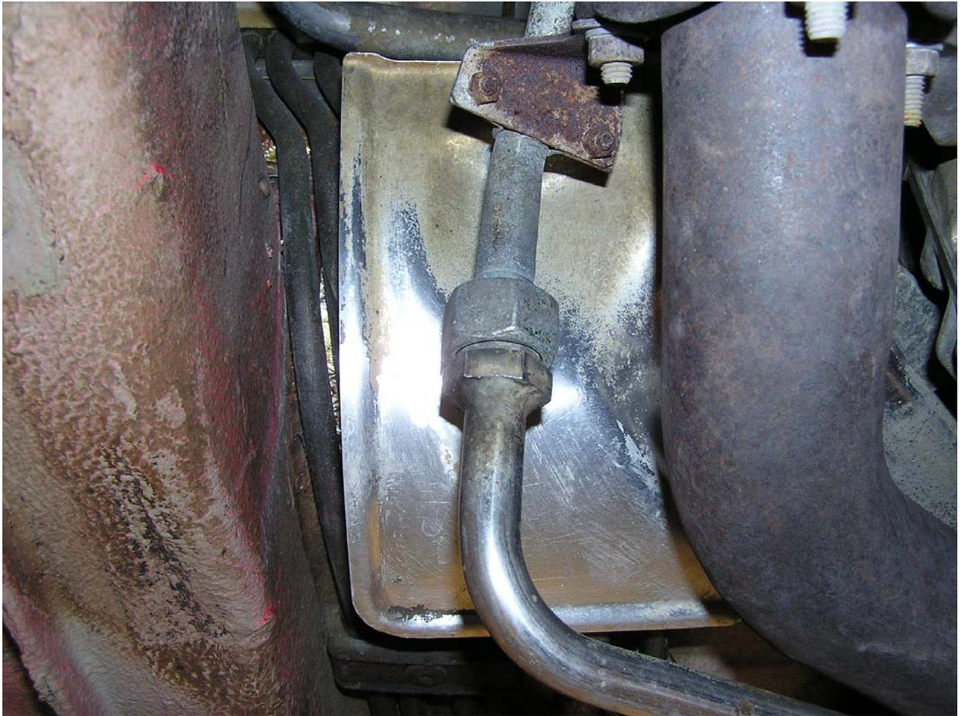
Remove rear clamps from factory catalytic converters. (15 or 17mm).
