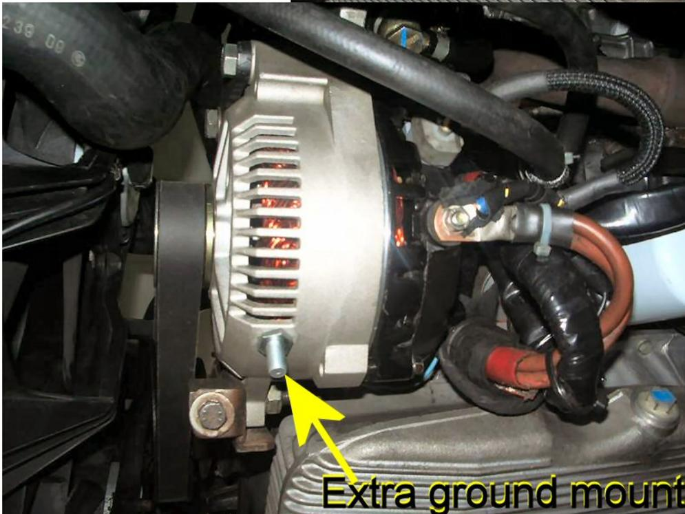
An extra ground mount has been provided on the alternator.
