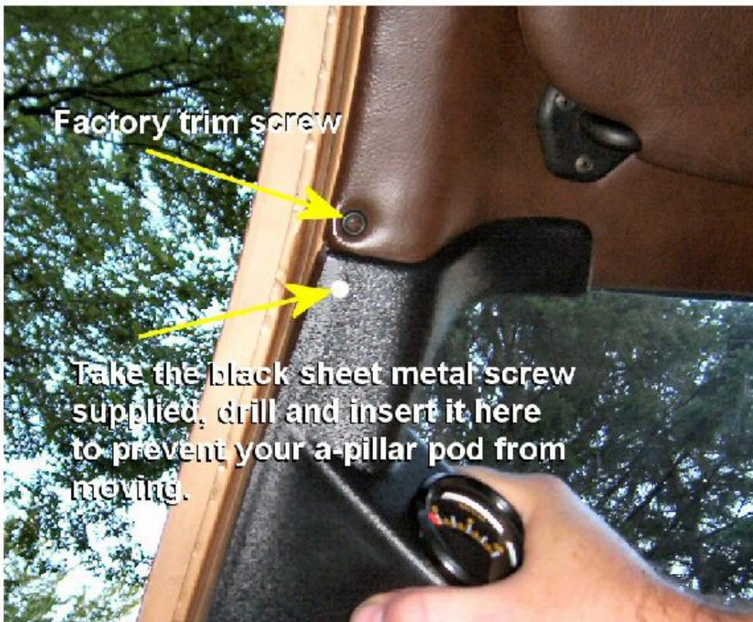
Take the black sheet metal screw supplied, drill and insert it here to prevent your a-pillar pod from moving.
