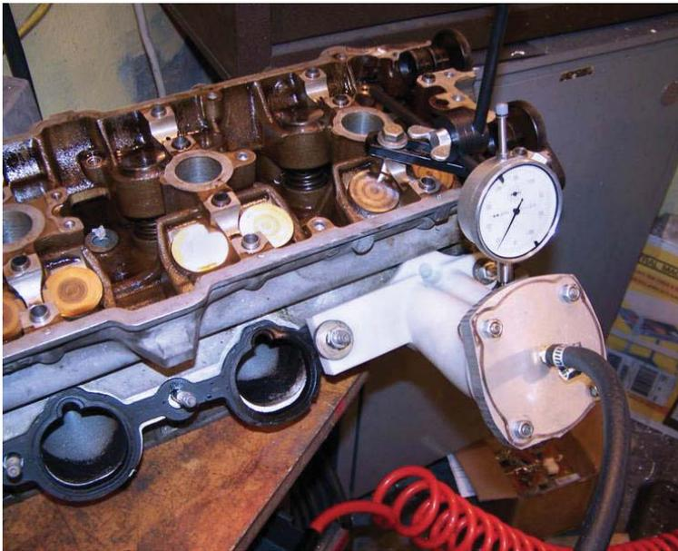
SLS Nylon 12 GF material was used to create the Porsche's intake runners. Here the SLS runner was attached to an actual engine cylinder head to test its heat resistance and strength.
