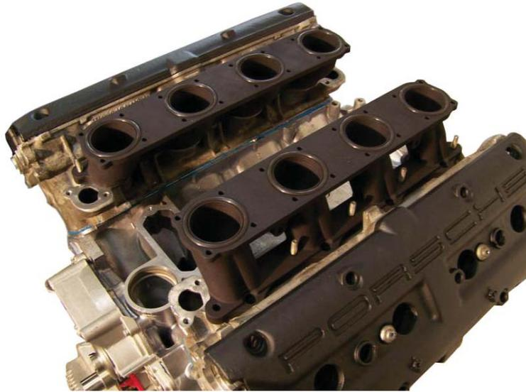
928 Motorsports LLC used functional SLS (Selective Laser Sintering) parts to complete their high-torque, Porsche 928 engine in an effort to enhance the air flow.
