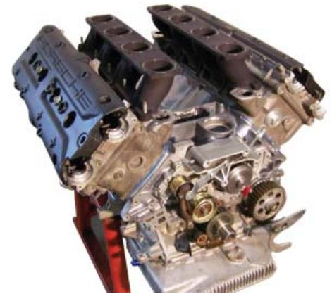
*With the help of Solid Concepts' SLS technology, 928 Motorsports experienced greater air flow for the 32-valve Porsche 928 engine.*
