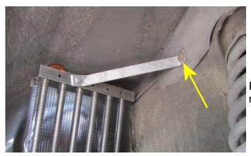
Remove the screw shown, slide the upper mount under it, and replace the screw.
