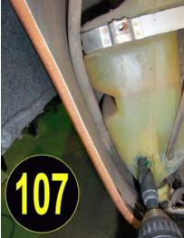
After we drilled a small pilot hole, take the proper bit for the tap you need for the fitting provided and drill out the remainder of the hole as shown in picture 107. The fluid in the windshield washer reservoir will drain down to the hole I just drilled, of course.
