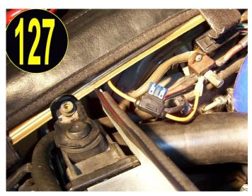
the fender to run your wire as shown in picture 128, and be sure to line the hole with the small grommet provided.
