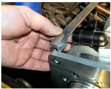
The front of the top strap is held to the supercharger bracket by a 40mm long Allen-head bolt supplied.
