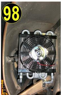
Your heat exchanger and fan assembly came shipped from 928 Motorsports, LLC. with the bottom mounting bracket and upper mounting bracket already attached. The U shaped mounting bracket and the inlet and outlet for the heat exchange
