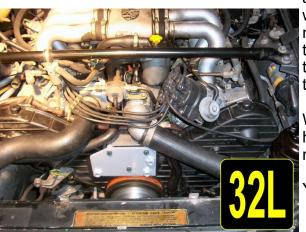
and machining in the 928 Motorsports mount, you will have to turn in each bolt several times and then move to the next bolt, turn it several times, move to the next bolt, turn it several times and so on, until the supercharger mounting plate is flush up against the motor before you can begin to torque them.
