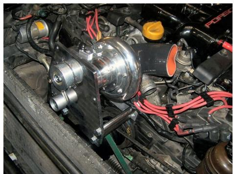
Put a drop of the Loctite blue on the threads of each of the 3 large mounting bolts.
