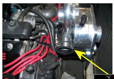
On Page 19 we placed the 2.5" black hose onto the outlet nipple of the Raptor, and added the two smallest T-bolt clamps to it. Your install should now look like this.
