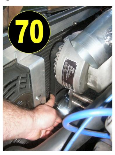
The front of your supercharger near the pulley should always be clean when you inspect it.
