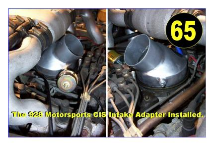
If your car is a US model, it will be equipped with a lambda sensor. It is going to have an air temperature sensing pipe that comes up to the intake manifold as shown in photo 61. If that is the case, you will need to install the 45 degree elbow into the CIS intake elbow to move the boost sensor up and out of the way of the lamda pipe.
