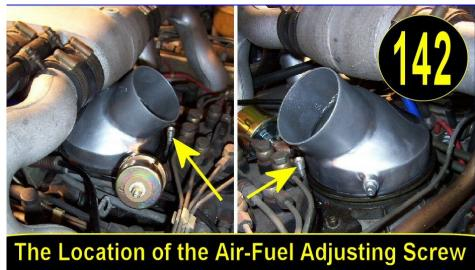
The adjusta 3mm allen socket located just between the CIS intake and he fuel distributor, as shown in picture 142. A very small adjustment has a rather large impact, so you want to be conservative with your adjustments. To turn the screw IN will RICHEN it, OUT will LEAN IT OUT. Your goal is a 11.5 or 12:1 air/fuel ratio at wide-open throttle.
