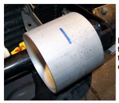
Find the 3" aluminum hose sleeve and draw a line in the center of it with a marker. It goes into the hose halfway—just up to the marker line, and is clamped with another #52 hose clamp.
