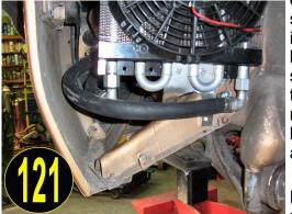
Earlier in these instructions, we attached the 9' long piece of heater hose t the bottom of the intercooler as we
