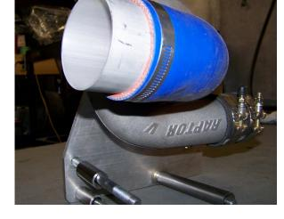
Now find the three inch length of 2 1/2" black hose and secure it to the outlet of the supercharger with one of the small T-blot clamps as shown. A second t-bolt clamp is placed on the hose also, but not tightened.
