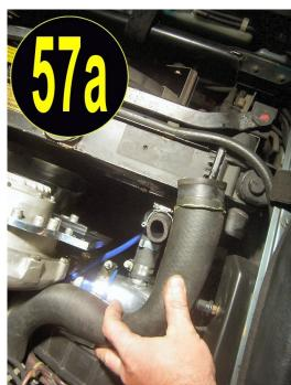
Trim about 1.5" from the end of your upper radiator hose and put it back on. See picture 57a. \*Note, the route of the finished upper radiator hose in picture 57b.
