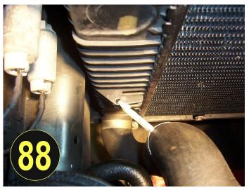
**Air Filter:** Now it's time to install the air filter assembly onto your supercharger kit. Take the K&N air filter with the intake elbow hose attached to it, as shown and slip the end over the intake elbow at the back of the supercharger head unit making sure you get it down and least 1/2" over the metal elbow and then clamp it. The air filter lays on top of the lower radiator hose and it is surrounded on all sides and is not clamped in place.
