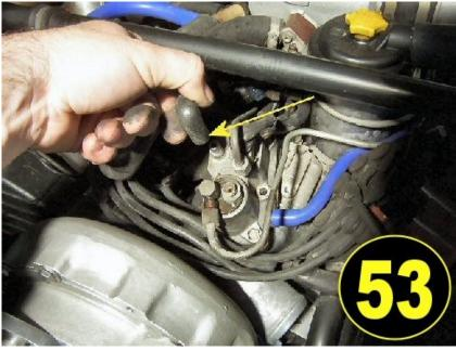
Photo 55 shows the warm up regulator now mounted vertically at the front of the motor like we want and that opens up the area we need for the air filter intake.. Later, when the supercharger is mounted, you can route your ignition wires like this:
