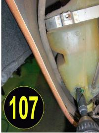
After we drilled a small pilot hole, take the proper bit for the tap you need for the fitting provided and drill out the remainder of the hole as shown in picture 107. The fluid in the windshield washer reservoir will drain down to the hole I just drilled, of course.
