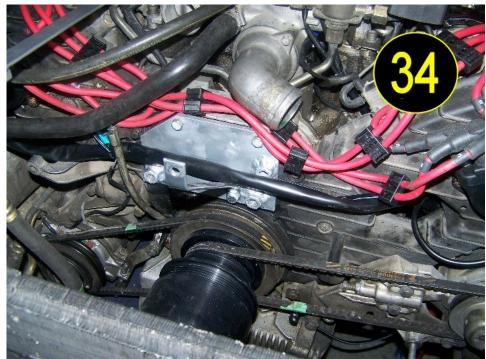
Take the Z-shaped support bracket from your kit and bolt it to the inner mount with the short 8x15mm bolt as shown in picture 34.
