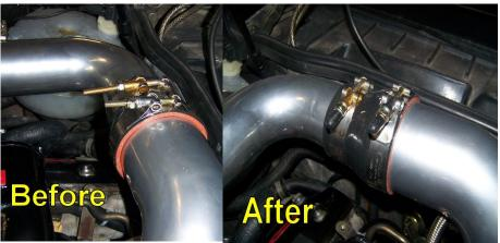
Place a shop towel or two beneath the bolts and use an airpowered cut-off tool, a hacksaw or even a bolt cutters to lop off an inch or so. Do not remove too much - your want to be able to remove and reinstall these clamps again in the future. Finish the ends of the bolts with a file to remove the burrs.
