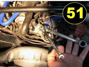
Save the two bolts and clean the threads on them because they will be reused. Now take a 10mm socket, and remove the remaining hex head bolt that mounts the warm up regulator to the top of the thermostat assembly. Then you can remove the triangular shaped adapter plate that was mounting your warm up regulator and we are now ready to turn the warm up regulator and mount it vertically back in the same position.
