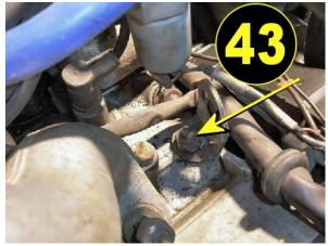
Locate and remove the engine lift hook located at the front of the right head, as shown in photo 43.
