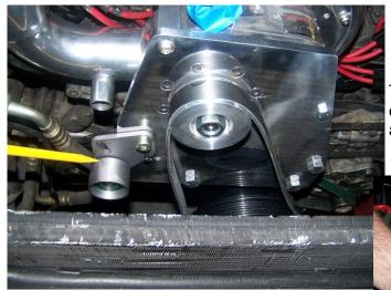
Insert a suitable pry bar over the bolt head and under the pin provided and pivot the tensioner to tighten the belt. Have a helper hold the pry bar in this position while you tighten the nut on the backside to hold it there. The head of the top bolt is extra tall so you can pry against it to adjust your belt tension as shown below.
