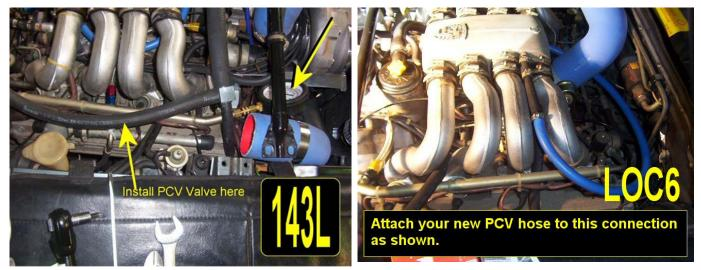
Install the PCV valve in this long 1/2" hose. Make sure you install it in the correct direction: so the air can flow *to* the intake manifold, but not *from* the intake manifold. Suck and blow on the PCV valve before installing it to learn which way to put it in.
