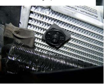
Locate all of the retainers before adding the retaining clips. You can tip the radiator top toward the engine to make this process easier.
