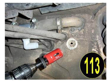
We cut a 1-1/8" hole as shown in picture 113 and then rounded it with the grommet provided so that the sharp edges would not cut our new water hose. See pictures 114 and 115. We cut a 1-1/8" hole because by the time we put a grommet around it to prevent chafing, a 3/4"
