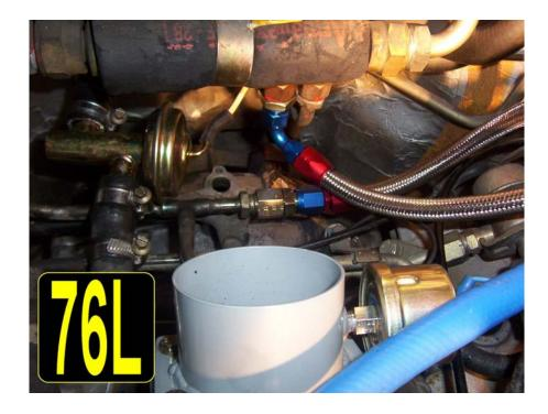
Use opposing wrenches to tighten every fitting. DO NOT OVER TIGHTEN. One of the first things we will do when we start the engine for the first time, is watch these fittings and check them for fuel leaks.
