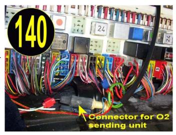
supercharger kit may need a oxygen sending unit for early cars and also those Euros that may not have an O2 sensor in the exhaust system. For those vehicles, the O2 sensing kit has to be installed in order for the gauge to function. Lets assume in these instructions that you already have a factory O2 sensor installed. (Call us if you need one)
