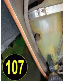
After we drilled a small pilot hole, take the drill bit that is sized for the tap you will use, and drill out the remainder of the hole as shown in picture 107. The fluid in the windshield washer reservoir will drain down to the hole I just drilled, of course.
