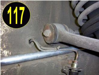
Remember, because we have the car in the air and the wheel off the car, the lower A-Arm is at its lowest most point as the caliper and break assembly is hanging completely down. That is very unusual and will never happen again unless the car goes airborne. Under normal circumstances, the upper A frame is even further from this conduit than it is at this time.
