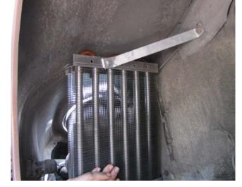
Remove the screw shown. Place the upper mount under it and replace the screw.
