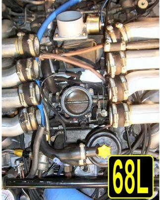
The easiest way to install it is to loosen all the clamps on your intake plenum, slide the rubber hoses out, and remove the center section. As shown in picture 68L. This makes installing the L-Jet clamp easy, and allows easy access to replace all your old vacuum lines while you are at it.
