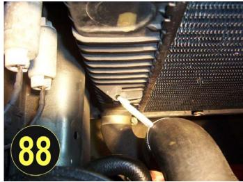
Now it's time to install the air filter assembly onto your supercharger kit. Take the K&N air filter with the intake elbow hose attached to it, as shown in photo 79L and slip the end over the intake elbow at the back of the supercharger head unit making sure you get it down and least 1/2" over the metal elbow and then clamp it. The air filter lays on top of the lower radiator hose and it is surrounded on all sides and is not clamped in place.
