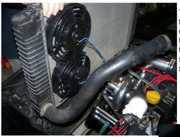
Take a look at the two 8" hi-volume electric fans included in your kit. They each have one flat side. They need to mounted so the flat sides face each other to fit on the radiator correctly. The top fan will have the flat side down, the lower fan will have the flat side up.
