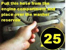
trim about 8 inches off the end, and stuff it behind the windshield washer reservoir. It will stay nice and dry and very safe back there, it is just a gas tank vent. Put your inner fender liner back on. Also, if you removed the air rail, go back and replace that bolt you removed on the fuel line support bracket a moment ago. (Photo 24).
