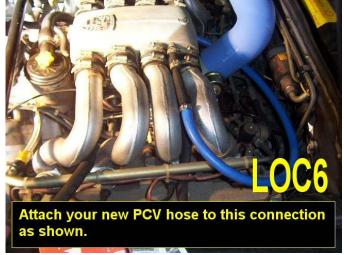
Install the PCV valve in this long 1/2" hose. Make sure you install it in the correct direction: so the air can flow *to* the intake manifold, but not *from* the intake manifold. Suck and blow on the PCV valve before installing it to learn which way to put it in.
