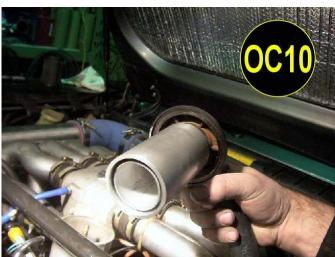
Now, disconnect the oil hose from the top of the oil separator to the intake manifold as shown in LOC1.
