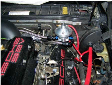
Now go back and tighten each fuel fitting with two wrenches in opposition.
