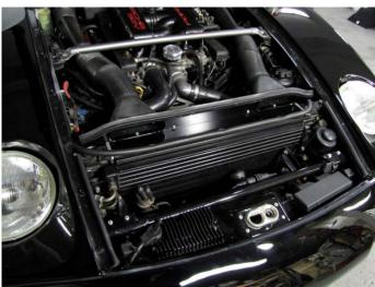
**Water-Wetter:** There is an additive called "Water-Wetter" that adds a surfactant to the water so it gets into greater contact with the uneven metal inside the motor, allowing it to transfer heat faster. It works. It will not fix a bad cooling system—but on an other-wise good cooling system that is struggling to keep up, it helps.
