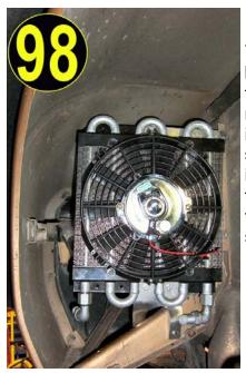
Your heat exchanger and fan assembly came shipped from 928 Motorsports, LLC. with the bottom mounting bracket and upper mounting bracket already attached. The U shaped mounting bracket and the
