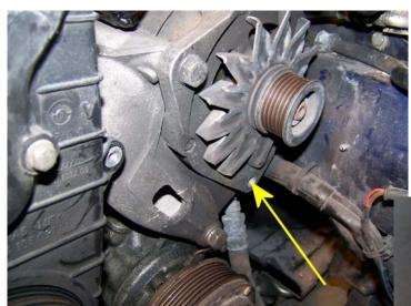
We can correct that by installing our 968 Idler Upgrade (provided) to increase belt wrap on the alternator.
