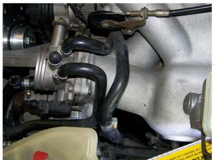
Route the finished hose down so that the end is near the steering rack.
