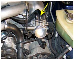
It is for this reason that the PCV hose has to be removed and re-routed to vent the crankcase to atmosphere.
