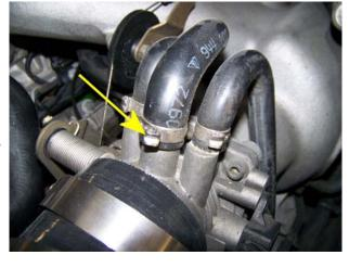
Cut the clamp with a wire cutters and remove it.
