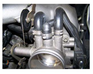
Install the cap provided and clamp it in place.
