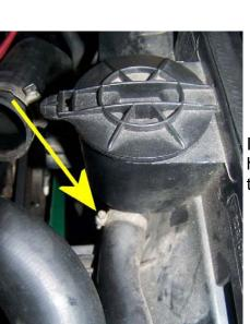
In the center of the fan shroud there may be a small air filter housing for the EGR system. Loosen the clamp and remove the hose that is attached to it.
