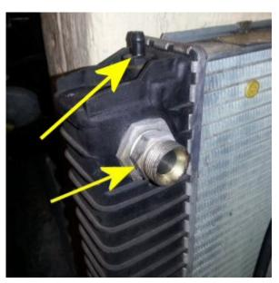
Check for debris trapped between the radiator and the AC condenser core. Hook up a shop vacuum and clean that out! It doesn't hurt to vacuum out the fins of the AC core, either. You will not have this good of access to it for a long time.
