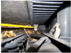
Lean the radiator toward the engine at the top to allow access to the fan switch found at the bottom front left end tank. Disconnect the wire connector from this fan switch.
