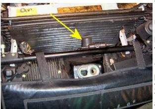
7) 1987-90 models with Moveable Grille Louvers: Porsche 928's from these years are equipped with moveable louvers operated by an electric motor to regulate air flow through the radiator. The system was known to cause over-heating when it failed, and they were discontinued by the factory in 1991.
