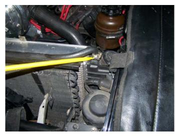
Bring the small radiator vent hose back over and attach it to the nipple on the left end tank now.
