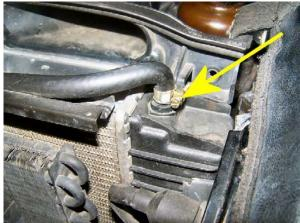
Loosen the clamp and remove the small vent hose from the top of the radiator end tank as shown here:
