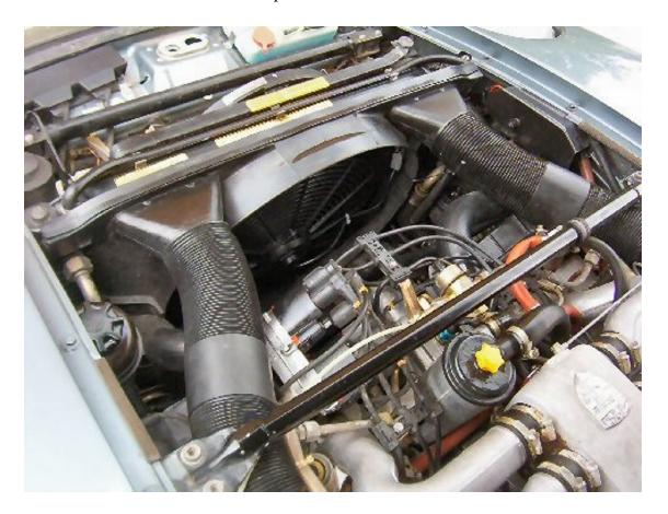
**TESTING THE INSTALL:** Start your engine. The new electric fan will not come on right away. It only comes on at 160 degrees F, and shuts off at temps below that also.
