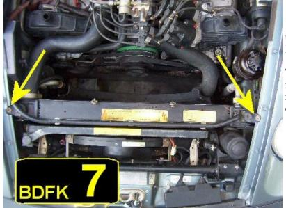
Remove the two 6mm Allen bolts from the upper radiator mounts as shown in Picture BDFK7.
