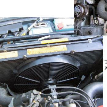
There is a flat spot in the shroud that should be placed on top as shown.
