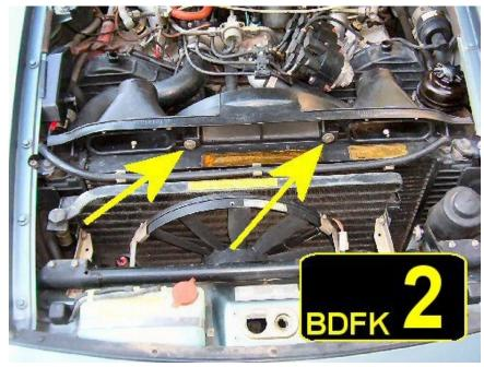
Remove two 10mm bolts at the top of the radiator, and lift off the upper radiator fan shroud.
