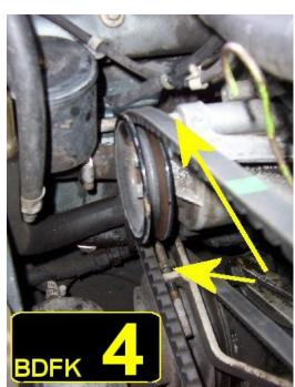
Loosen and remove the Air Pump/Fan belt. Two 13mm bolts, and loosen the nut on the threaded adjuster if you have one.
