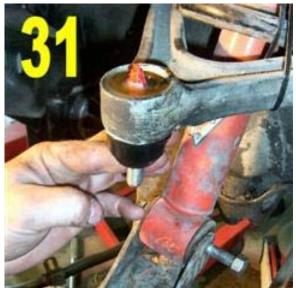
Then rotate the ball joint pin back and forth and let the new boot find it's final resting place. You should discover the new joint is quite stiff, but is able to pivot when you move it by hand.
