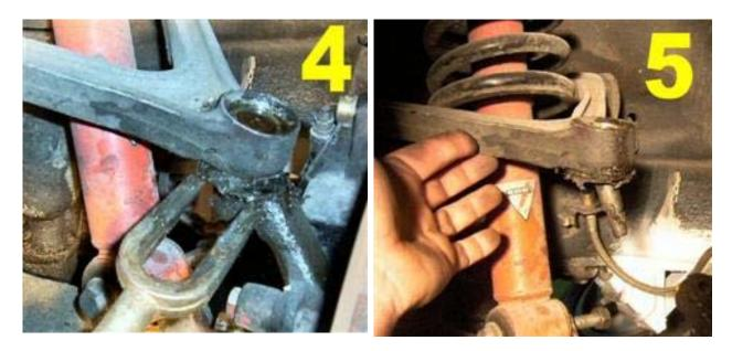
If you did raise the spindle in Step 3 making it easier to get at the nut and loosen it, remove the jack from the rotor so that the suspension is completely unloaded. That will facilitate breaking the ball joint free.
