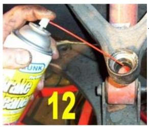
A shot of carb spray or break cleaner will do a nice job at cleaning out the inside of the socket making sure that any grit or sand remaining in that socket is washed out before we start reassembling it.
