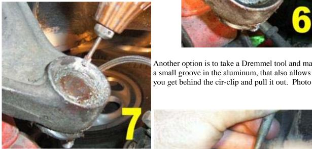
This will also facilitate you reinstalling the cir-clip later. This entire cup will be sealed with epoxy when we finish, so the small cut you make with the Dremmel tool will not cause any harm.
