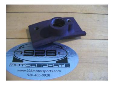
By installing our Crank Reference sensor Adapter, an early K-Jet or L-Jet equipped engine can be adapted to hold a crank reference sensor. This allows early engines to upgrade to the later LH-Jetronic or Electromotive Tec GT engine management systems.
