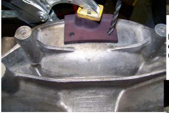
Tap the holes, and insert the M6 bolts with washers provided. Do not over-tighten!
