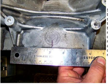
Start by measuring the distance between the two uprights as shown and mark the middle of the block between them. Try to be accurate, but don't worry too much about it if you are using our Tec GT Engine Management System because you can add or remove degrees from the crank in the software as needed.
