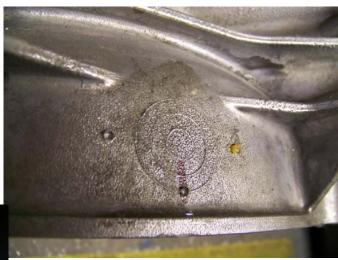
Drill the two outer mounting holes with the recommended drill bit for your M6 x 1.0 bolts (provided)
