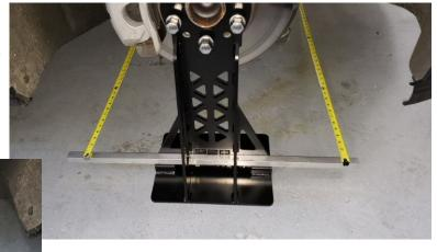
The distance between the two tape measures should be about the height of the tire.
