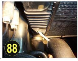
that it doesn't get cut. You do not need to pull it away hard, this is just to keep the hose from going **in** toward the motor.
