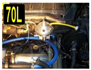
Take the fuel management unit now and hold it up on the firewall and mark the holes where you are going to drill to mount the mounting bracket. Make sure you locate it low enough to allow the hood to close and within reach of the fuel lines we will be adding as in picture 74L and 75L. The mount bracket is shown in picture 71L.
