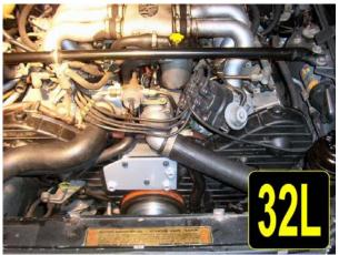
Washers are not necessary underneath the bolt heads as we used washered bolts that do not require separate washers. Torque to 25 ft. lbs.
