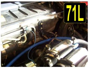
picture 71L and 70L. After the bracket is mounted, go ahead and mount the FMU on the bracket as shown in picture 70L. Then install the 1/4" NPT to 6-AN adapters into the FMU as shown.
