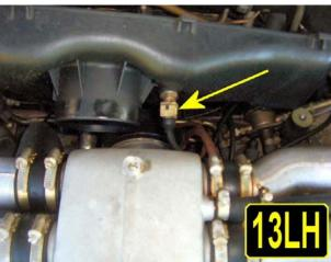
As you lift up the air filter box, unclip the air temp sensor shown in picture 13LH.
