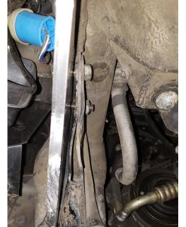
Your new protection plates get mounted to the OUTSIDE of each of the factory tie-down brackets, and must be pointed reasonably (not perfectly) straight forward.
