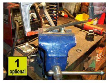
Put a 25mm socket around the outside of the assembly and begin turning it in. If you place the socket all the way up to touching the pan as in Picture 1 below, that will help you keep the assembly going straight in while you turn it.
