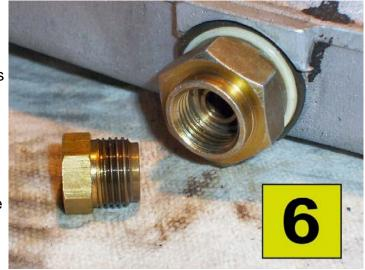
The finished drain plug is equipped with a special inverted flare. You do not have to torque it as tight as you are used to, and it will not leak.
