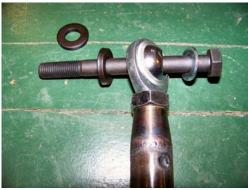
Tighten the bolts on both ends loosely.
