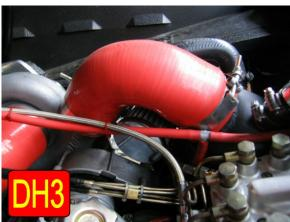
We "clocked" the outlet of the supercharger for you in what should be the right location. if you should find that the outlet needs to be rotated a little bit. loosen the allen-head screws around the super-
