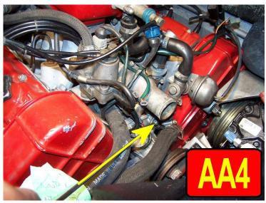
You'll find that removing the Aux Air valve opens up a vacuum nipple on the central intake plenum — this is where you hook up the vacuum hose to the blow-off valve as shown in picture D5.
