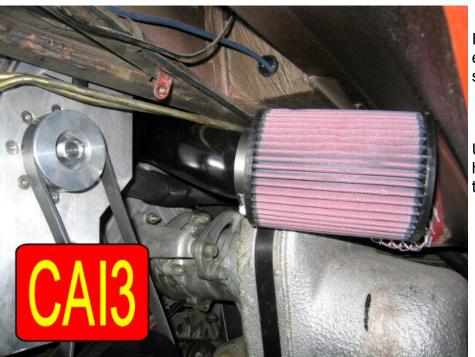
Install the air filter onto the end of the cold air intake as shown in CAI3
