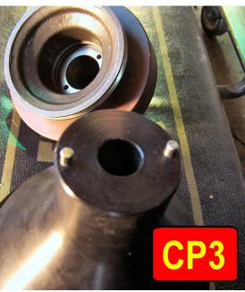
Have your assistant lock the engine again with the screwdriver in the clutch inspection slot as before, (Picture CP1) and tighten the crankshaft pulley bolt to 218 ft lbs of torque.
