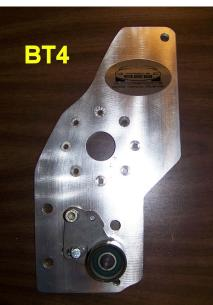
Hold your belt tensioner up to your supercharger mounting bracket and find the best setup for your car.
