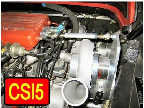
Put a ring of the same silicone around the base of the CSI where the o-ring is, and slide it onto the studs WITH THE ELECTRICAL CONNECTION FACING UP. Install the two mounting nuts and tighten. Refer to pictures CSI 4, 5, and 6. Finish by attaching the electrical connector and tightening the fuel line banjo bolt.
