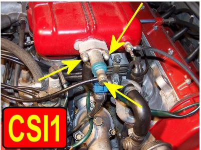
Then remove the two 10mm nuts the hold the CSI to the intake manifold center plenum as shown.
