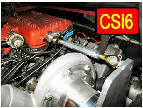
Pictures CSI5 and CSI6 show the Tracking Turnbuckle attached to this CSI mount. Do not install the Tracking Turnbuckle at this time, we will do that after the supercharger is mounted.
