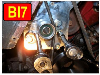
There is also a pin provided in your belt tensioner bracket so that you may insert a screwdriver between the swing-bolt and the pin and pry to tension the belt.
