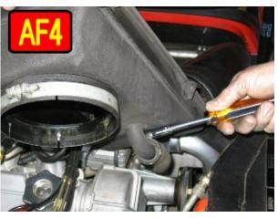
Keep track of the small hose you disconnect from the bottom of the air filter cover as in AF4. We will be looking for that hose again to re-attach it to the new cold air intake.
