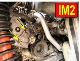
We can now install the steel inner supercharger mount. Locate the inner supercharger mount, spacers, and the two long metric mounting bolts from your kit (Picture IM3) and mount them according to the belt system you have on your vehicle as follows:
