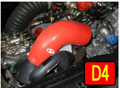
Locate the blow-off valve assembly, the pre-molded 3/4" hose and two clamps as shown in Picture D4 and D5, and mount them to the Diffuser you just installed. The BOV and the breather fit under the intake elbow as shown so the bonnet will close correctly.
