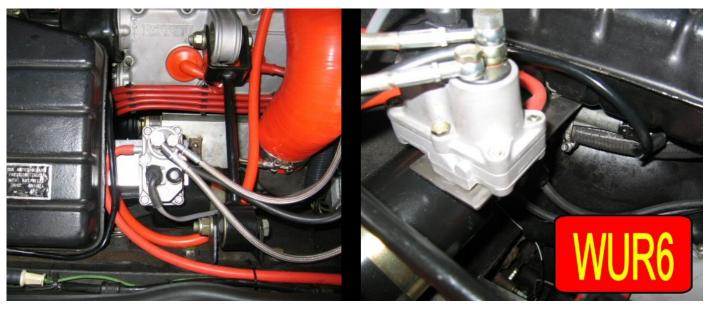
are no kinks in them, and re-tighten the fuel line fitting on top of the WUR.
