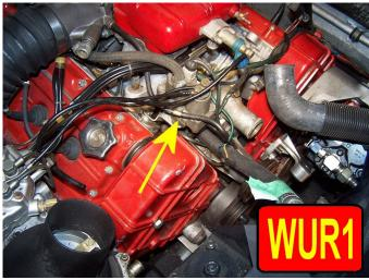
We need to re-position the Warm-Up Regulator the item shown in Pictures WUR1 and WUR2. We will be relocating it over by the radiator coolant tank as shown in Picture WUR3 and mounting it there with the custom mounting bracket provided as shown in Picture WUR4.
