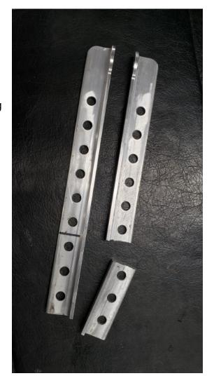
In this picture, the Seat Mounts have been shortened and it is ready for installation.
