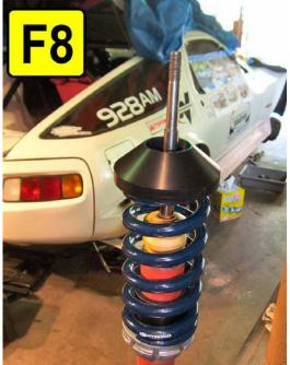
Referring to picture F2, (previous page) slide the stainless steel spacers on to the shocks now, in place of the old plastic dust boot part #6..
