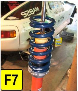
Then take the front spring and slide it down on top of the adjuster nut which will serve as the spring perch and over the outside of the center adaptor that we just installed. See photo F7.
