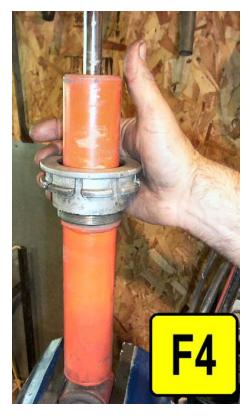
Then take the 928 Motorsports adapter collar and slide it down over the Koni. This centers the coil spring so that it cannot shift from side to side. Photo F5.
