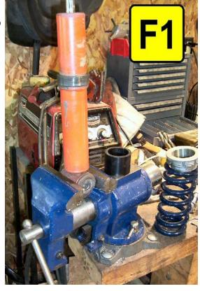
Clamp the shock in a bench vise as in photo F1. It bears noting that you <u>never ever</u> clamp a shock absorber on the outside cylinder wall as the piston runs just inside that wall and any dent in that orange tower on the Koni would destroy the shock absorber. As you can see, you only clamp the shock absorber in a vise at the mounting base.
