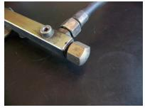
Be careful not to lose the metal ball inside the cap! Save the cap and ball in a bag for later in case you ever want to put them back on.
