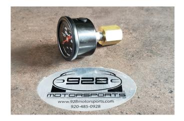
The following pictures show the installation of the fuel pressure gauge with the fuel rail on a workbench for clarity. There is no need to remove the fuel rail from the car to install the gauge.
