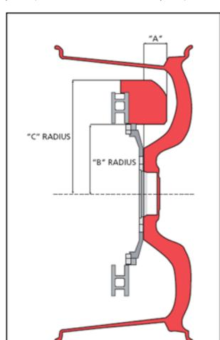
All measurements are taken from the back side of the wheel hub, with the wheel off. Use the center point of the wheel to measure. Brembo recommends a minimum of 3mm clearance between the caliper and the wheel spoke or rim.
