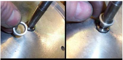
This shim will be under your old impeller and it goes back on with our impeller also. Remove all the small, thin shims.
