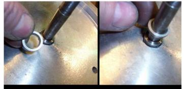
The shims are added beneath your impeller as shown.
