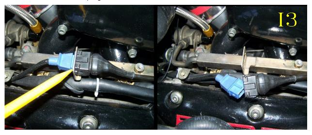
Disconnect the fuel lines on each end with 19MM and 15mm wrenches . Always use two wrenches in opposition whenever possible.
