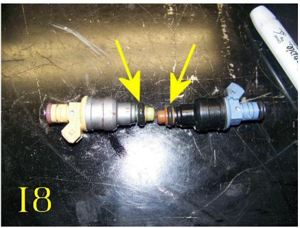
Install the new injectors, attach the connectors, add the fuel rail to the top and lock it down with the 10mm bolt you removed in Step 15. Add the fuel lines to each end, but do not install the top cover yet.
