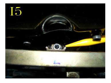
Pull up on the fuel rail and wiggle it, until it comes off the top of the 4 injectors on this side.
