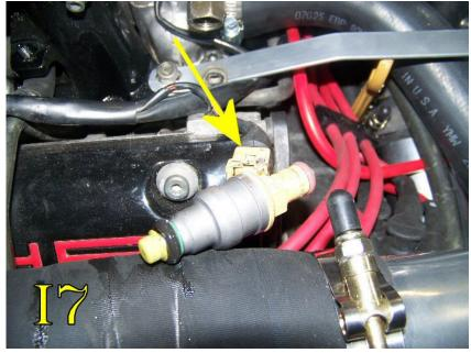
Compare the O-rings between the injectors you just removed and the new injectors. If your injectors have larger O-rings (as shown in picture 18) simply transfer those O-Rings onto the new injectors.
