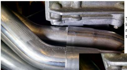
These pictures show the modified lower bell housing back on the motor, and the headers are installed with plenty of clearance.
