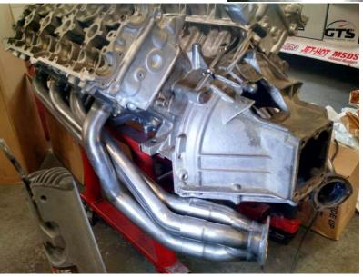
You may put the modified lower bell housing back on with only 4 of the original 6 fasteners. It is just a dust cover, and 4 bolts are a great plenty to hold it in pace.
