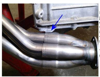
In these pictures, the engine is out of the car just for photographic purposes. The flange on the lower bell housing can be removed with the lower bell housing in the car, but as it is held on simply with only 6 fasteners, it is very easy to take off so you may modify it on the workbench.
