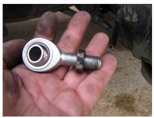
Remove the jam nut from the old tie rod end and thread it on to the new tie rod end.
