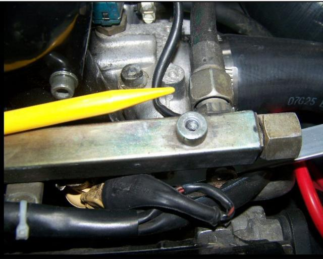
Use a 10mm socket to remove the two nuts that hold the fuel rail down to the manifold. These nuts are located behind the fuel rail—on the intake manifold side.
