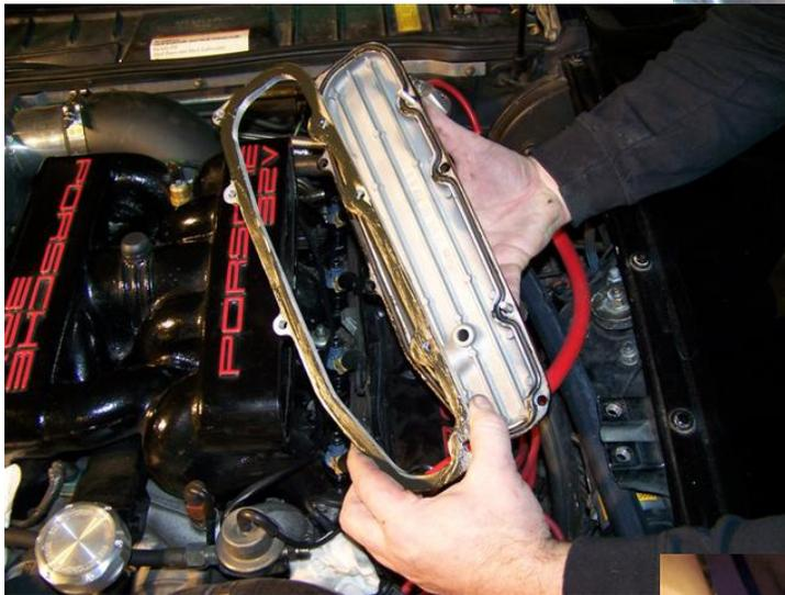
Using the gasket sealant provided in your kit, put a film of sealant on the side of the spacer that faces the manifold.
