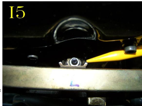
If the fuel rail has not been removed in a long time, you will be surprised how tight it can be seated! Lift off the fuel rail, and set it to the side.
