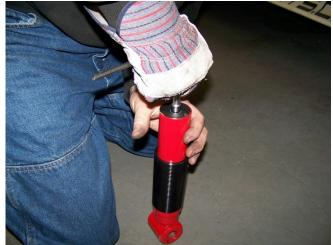
Continue pressing down and turn the valve clockwise gently until you have gently closed the valve. Note the direction your wrench is pointing, and open the valve (counter-clock-wise) 1 full turn (360 degrees) if it's a front shock; and 1.5 turns (540 degrees) if it's a rear shock. Let go, and the shock will slowly rebound up. They are adjusted and ready to install now.
