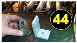
You will remove the engine lift hook located at the front of the right head, as shown in photo 43.
