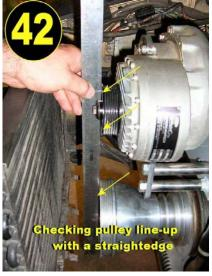
Now that we have mounted the supercharger head unit to the motor, we're going to take a straight edge across the crankshaft pulley and see if it lines up with the front of the supercharger pulley. They have to be perfectly in the same plane. See photograph 42.
