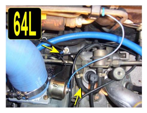
Also, notice the arrow in picture 64L pointed at the black rubber return fuel line coming out of the fuel pressure regulator in that picture.
