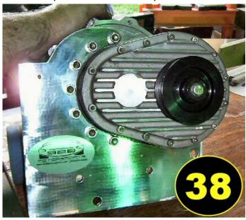
These are grade 8 aircraft quality bolts, extremely strong. Slide them through the forward mount of the supercharger bracket and slide the spacers on the back of them, as shown in photo 40.
