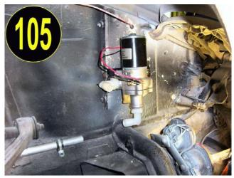
We don't use bolts and nuts because the other side f the fender well is not available to us, and we can't use sheet metal screws because they penetrate too far and also sheet metal screws vibrate loose over time. So these steel rivets are a good way to go. You will use two or three rivets on the right hand side of the water pump when you mount it to the fender well and you will use one or two rivets on the 90 degree L-shaped angle on the left side as shown.
