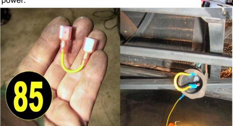
After the wires are routed, you can test this circuit by turning the key on. When you turn the key to the "run" position all three electrical fans should operate. Then loom the wires together with cable tied again to prevent them from working loose or getting into a belt or mechanism and getting pinched. Looking at photo 86 you can see the completed wiring for the fans and how it is loomed up tight against the bottom of the car, being secured and out of harms way.
