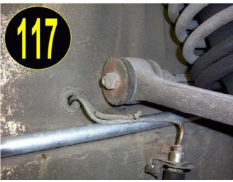
Remember, because we have the car in the air and the wheel off the car, the lower A-Arm is at its lowest most point as the caliper and break assembly is hanging completely down. That is very unusual and will never happen again unless the car goes airborne. Under normal circumstances, the upper A frame is even further from this conduit than it is at this time.
