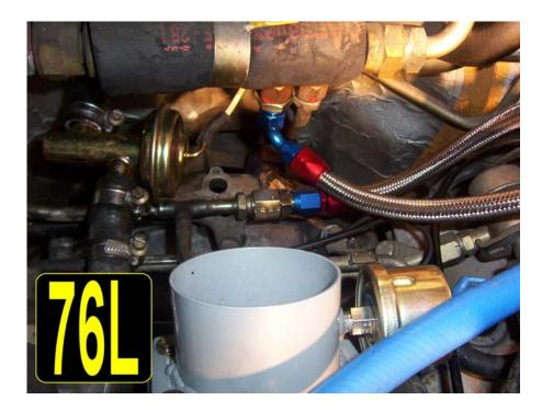
Use opposing wrenches to tighten every fitting. DO NOT OVER TIGHTEN. One of the first things we will do when we start the engine for the first time, is watch these fittings and check them for fuel leaks.
