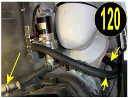
Now, please take the 7' long piece of 3/4" heater hose and the long, heavy red wire supplied and fasten the ends of them together with some electrical tape (temporarily).
