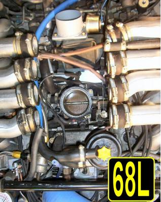
The easiest way to install it is to loosen all the clamps on your intake plenum, slide the rubber hoses out, and remove the center section. As shown in picture 68L. This makes installing the L-Jet clamp easy, and allows easy access to replace all your old vacuum lines while you are at it.
