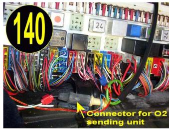
the bottom. Your 928 Motorsports, LLC supercharger kit may need a oxygen sending unit for early cars and also those Euros that may not have an O2 sensor in the exhaust system. For those vehicles, the O2 sensing kit has to be installed in order for the gauge to function. Lets assume in these instructions that you already have a factory O2 sensor installed. (Call us if you need one)
