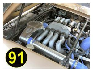
The direction of the coolant flow in this system is optimal and has been designed to use as few running feet of hoses as possible. Hot air will enter the intercooler and cold air will exit the intercooler. The hot air will give off it's heat into the water with-in the intercooler.
