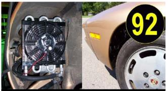
On the Stage 2 kit, we mount our heat exchanger for the intercooler system behind the left headlight not in front of the engine radiator. This helps run both the intercooler and the engine cooler - as the radiator is not being blocked or fed warm air.
