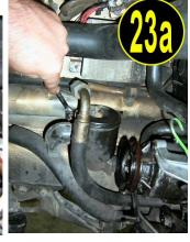
Now we have the air pump assembly removed and all the lines have been plugged, the crank shaft pulley is removed and all the belts obviously with it, and the air filter air box has been removed and its mounts. We have completed the disassembly portion of the installation. This is a good time to clean the engine up a bit before we begin the assembly of actually installing the supercharger kit to the motor.
