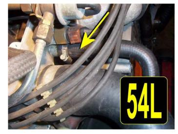
We recommend that you coat these bolts with loctite red which you will find in your kit, to keep them from backing out. You may want to clean up the threaded holes in your motor with a metric tap if you see signs of corrosion before proceeding. Because of the precise drilling and machining in the 928 Motorsports mount, you will have to turn in each bolt several times and then move to the next bolt, turn it several times, move to the next bolt, turn it several times
