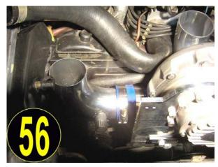
After the 3" blow-off valve elbow is properly positioned and pointing straight up in front of the right camshaft tower, you can now tighten the 7/16" hex head bolts that go around the perimeter of the head unit to hold the head unit in that position. (See photo 49).
