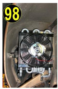
Your heat exchanger and fan assembly came shipped from 928 Motorsports, LLC. with the bottom mounting bracket and upper mounting bracket already attached. The U shaped mounting bracket and the inlet and outlet for the heat exchanger are at the bottom. Place the heat exchanger assembly on top of your fender strut so that the U shaped bracket straddles it with a leg on each side. As shown in picture 98.
