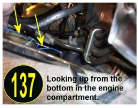
Pull enough through so that it reaches the boost pressure sending unit that you previously installed in your CIS intake elbow. You can go ahead at this time and put a ring terminal connector on it and mount it to the boost sender. You want to wire tie the wire up and away to make it look attractive and also kept it from contacting any hot exhaust manifold.
