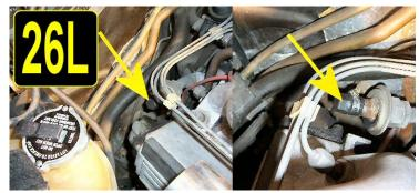
EGR OPTION 2: Leaving the air rail and capping it. Install 3/4" caps as shown in Picture
