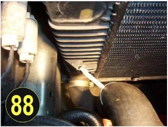
Now it's time to install the air filter assembly onto your supercharger kit. Take the K&N air filter with the intake elbow hose attached to it, as shown in photo 79 and slip the end over the intake elbow at the back of the supercharger head unit making sure you get it down and least 1/2" over the metal elbow and then clamp it. The air filter lays on top of the lower radiator hose and it is surrounded on all sides and is not clamped in place.
