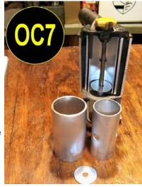
If the baffle on the inside of your OEL cap is so long it covers the holes in our inner baffle, shorten it with a hacksaw to just above our air holes in the center baffle.
