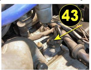
Replace the engine lift hook with the upper mount as in photo 45, with the same bolt and washer. **Do not tighten it down at this time.**
