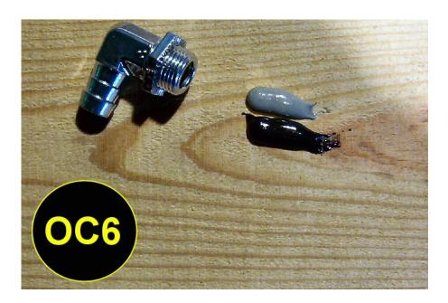
Make sure that the barbed hose nipple point straight up when you're done. This will have to set 1 hour before we can use the nipple so we will move on to another project and come back to this after the epoxy has hardened. We use the J.B. Weld epoxy specifically because of it's ability to withstand high temperatures and also oil. It is not softened by oil or temperature. While we wait for that to harden, lets move on to the oil separator itself.
