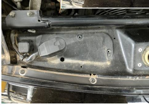
2) Remove the mounting bolts and the amplifier from the car.
