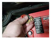
5) Then place these ring terminals on the threaded post on the left side, as shown.
