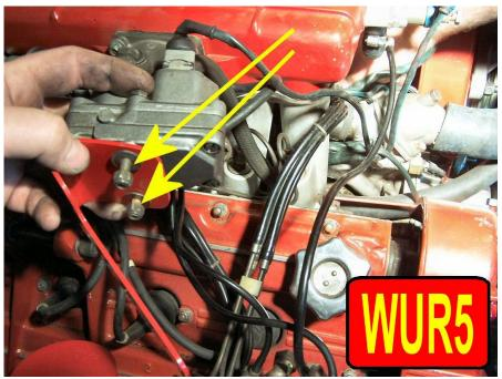
Mount the assembly back onto the intake manifold and put the 13mm nuts back on, as shown in WUR6. Leave the lower nut loose for the moment – we need to get under that again soon.
