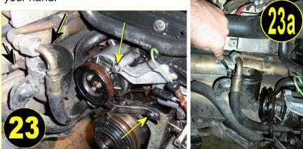
Now we have the air pump assembly removed and all the lines have been plugged, the crank shaft pulley is removed and all the belts obviously with it, and the air filter air box has been removed and its mounts. We have completed the disassembly portion of the installation. This is a good time to clean the engine up a bit before we begin the assembly of actually installing the supercharger kit to the motor.
