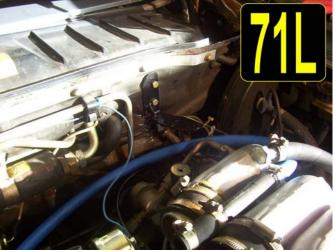
picture 71L and 70L. After the bracket is mounted, go ahead and mount the FMU on the bracket as shown in picture 70L. Then install the 1/4" NPT to 6-AN adapters into the FMU as shown.
