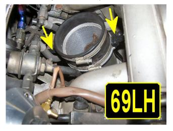
Now take the clamps we cut of in picture 65LH and slide them down the straps and tight up against the MAF, as shown in picture 70LH.
