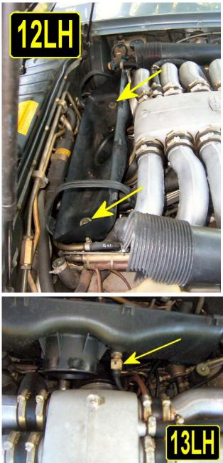
As you lift up the air filter box, unclip the air temp sensor shown in picture 13LH.
