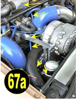
If your car is an automatic, you will be installing a T there instead in the vacuum line that comes out of the very same fitting. Take a vacuum hose from the kit of blue silicone vacuum hoses provided and run it from the intake manifold nipple or tee to the connection on the bottom of the blow-off valve. A cable-tie will keep it up near the radiator hose and away from the belts. See photo 67a.
