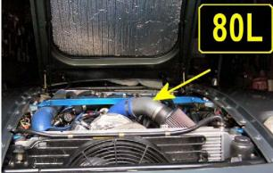
Check the installed height to make sure it is not too high for the hood to close as in picture 80L.
