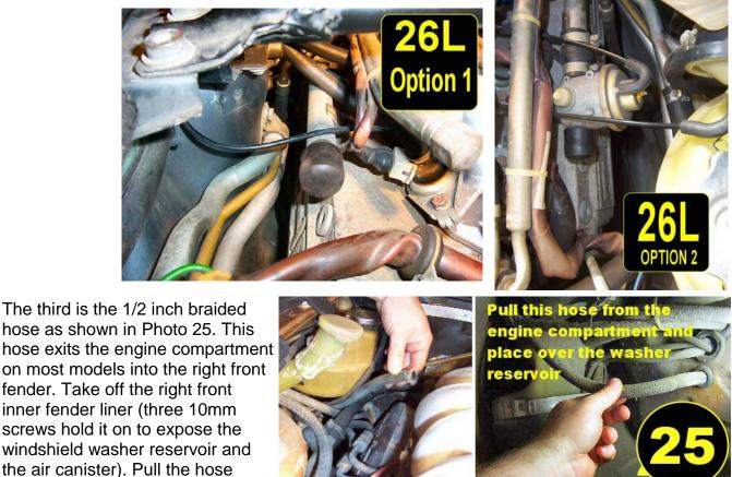
trim about 8 inches off the end, and stuff it behind the windshield washer reservoir. It will stay nice and dry and very safe back there, it is just a gas tank vent. Put your inner fender liner back on. Also, if you removed the air rail, go back and replace that bolt you removed on the fuel line support bracket a moment ago. (Photo 24).
