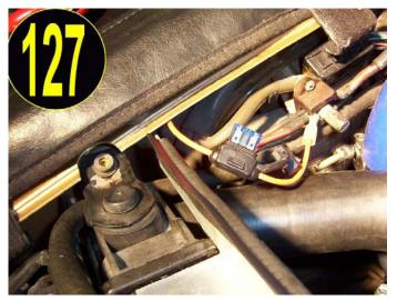
Drill the fender to run your wire as shown in picture 128, and be sure to line the hole with the small grommet provided.
