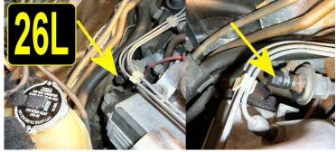
**EGR OPTION 2:** Leaving the air rail and capping it. Install 3/4" caps as shown in Picture 26L Option 1 and 26L Option 2.
