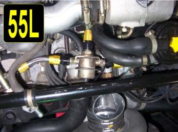
Install the braided fuel lines with the metric fittings as shown in pictures 56L and 57L.
