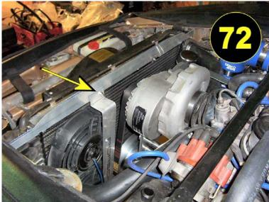
Next, remove the rubber gasket from the top of the old fan shroud, see photo 73 and carefully place it on top of your new aluminum 928 radiator shroud, so that the end products looks like photo 74LH.
