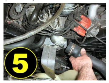
Disconnect the oil lines to the radiator (if you have them) – always using two wrenches in opposition to loosen the lines so you do not break the radiator nipples! Then you can remove the 6MM hex-headed bolts that secure the rubber hold-down clamps (photo 6) on each side of the radiator, and pull the radiator out thru the top.
