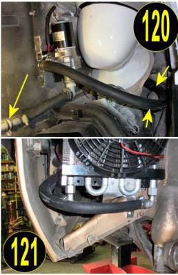
Now, please take the 7' long piece of 3/4" heater hose and the long, heavy red wire supplied and fasten the ends of them together with some electrical tape (temporarily).
