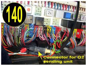
supercharger kit may need a oxygen sending unit for early cars and also those Euros that may not have an O2 sensor in the exhaust system. For those vehicles, the O2 sensing kit has to be installed in order for the gauge to function. Lets assume in these instructions that you already have a factory O2 sensor installed. (Call us if you need one)
