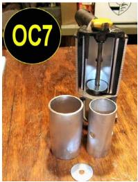
If the baffle on the inside of your OEL cap is so long it covers the holes in our inner baffle , shorten it with a hacksaw to just above our air holes in the center baffle.
