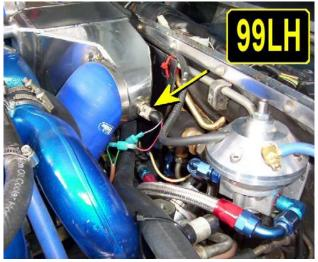
Drill the intercooler where you marked it, tap it, and set the temp sender into that hold with a little JB Weld on the threads to seal it as in photos 100LH and 101LH.
