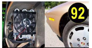
On the Stage 2 kit, we mount our heat exchanger for the intercooler system behind the left headlight not in front of the engine radiator. This helps run both the intercooler and the engine cooler - as the radiator is not being blocked or fed warm air.
