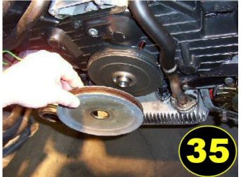
Now, remove the locking tool from the flywheel if you installed one, and replace the clutch slave cylinder and push rod.
