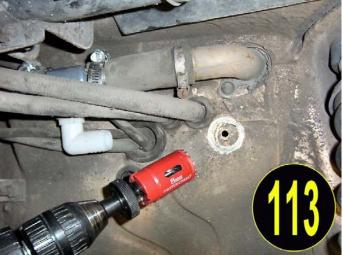
We cut a 1-1/8" hole as shown in picture 113 and then rounded it with the grommet provided so that the sharp edges would not cut our new water hose. See pictures 114 and 115. We cut a 1-1/8" hole because by the time we put a grommet around it to prevent chafing, a 3/4" water line is going to run perfectly through that grommeted area.
