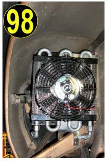
Your heat exchanger and fan assembly came shipped from 928 Motorsports, LLC. with the bottom mounting bracket and upper mounting bracket already attached. The U shaped mounting bracket and the inlet and outlet for the heat exchanger are
