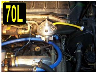
Take the fuel management unit now and hold it up on the firewall and mark the holes where you are going to drill to mount the mounting bracket. Make sure you locate it low enough to allow the hood to close and within reach of the fuel lines we will be adding as in picture 74L and 75L. The mount bracket is shown in picture 71L.
