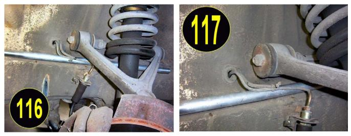
Remember, because we have the car in the air and the wheel off the car, the lower A-Arm is at its lowest most point as the caliper and break assembly is hanging completely down. That is very unusual and will never happen again unless the car goes airborne. Under normal circumstances, the upper A frame is even further from this conduit than it is at this time.
