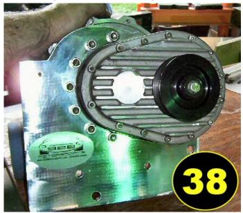
These are grade 8 aircraft quality bolts, extremely strong. Slide them through the forward mount of the supercharger bracket and slide the spacers on the back of them, as shown in photo 40.
