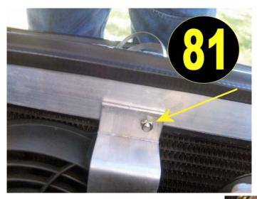
The left side of the fans are secured to the radiator core with the black cable ties provided. Put them through the mounting holes in the fans and forward through the radiator to the front, then bend them back over a cross-tube and send them back through the radiator to connect at the back. Photo 84. Then trim the extra off with the snipers.
