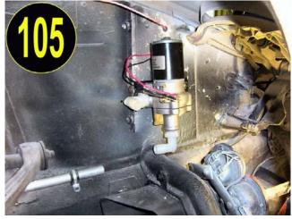
We don't use bolts and nuts because the other side f the fender well is not available to us, and we can't use sheet metal screws because they penetrate too far and also sheet metal screws vibrate loose over time. So these steel rivets are a good way to go. You will use two or three rivets on the right hand side of the water pump when you mount it to the fender well and you will use one or two rivets on the 90 degree L-shaped angle on the left side as shown.
