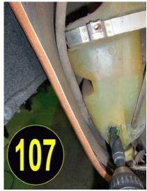
After we drilled a small pilot hole, take a 3/4" drill bit, and drill out the remainder of the hole as shown in picture 107. The fluid in the windshield washer reservoir will drain down to the hole I just drilled, of course.
