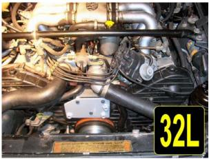
Washers are not necessary underneath the bolt heads as we used washered bolts that do not require separate washers. Torque to 25 ft. lbs.
