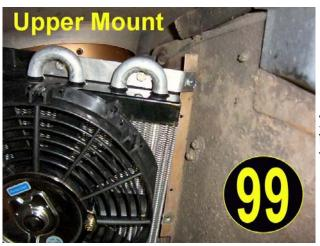
In picture 99 we're taking one of the screws that you just removed when you took off the inner fender liner and putting it back in the upper mount to hold the heat exchanger in place on top.
