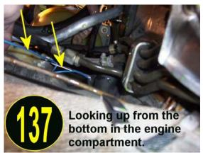
Pull enough through so that it reaches the boost pressure sending unit that you previously installed in picture 137LH. You can go ahead at this time and put a ring terminal connector on it and mount it to the boost sender. You want to wire tie the wire up and away to make it look attractive and also kept it from contacting any hot exhaust manifold.
