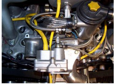
While you have the oil breather assembly off, take a flashlight and look straight down into the motor. You'll see how easy it is for the crankshaft counterweights to sling oil up into your breather system without this baffle plate!
