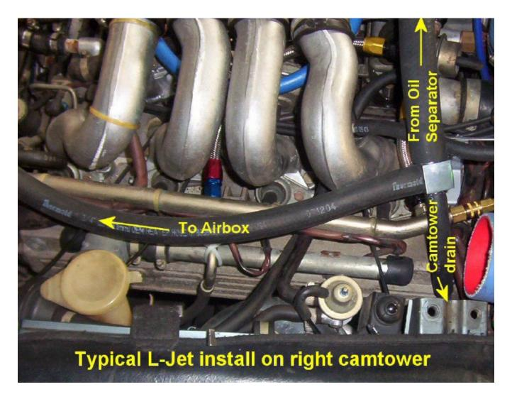
Instructions for installing the drain elbow are on the following page.
