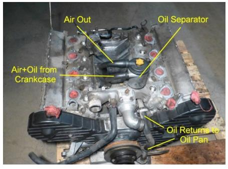
**How it Works:** Crankcase fumes wet with motor oil exit the top of the motor via the vent housing connected to the engine block. These Air/Oil Fumes enter the Oil Separator at the side, where they spin around, throwing the oil against the outer wall of the separator. The gases exit the top of the oil separator, and the oil that collects in the bottom is returned to the oil pan via a hose that runs under the water bridge down the front of the motor.
