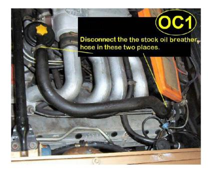
Once you have both ends disconnected, you will discover that there is some small water lines that go through that oil breather hose to warm it as shown in **picture OC2**
