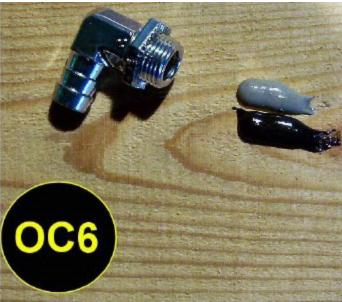
As in **OC6**, layout two equal-sized stripes of the J.B. Weld metallic epoxy, on e of the hardener and one of the liquid metal. Then mix them together to where they become a consistent gray color. Coat the threads of the cam tower barbed nipple as shown in **OC6** and screw it into your cam tower.
