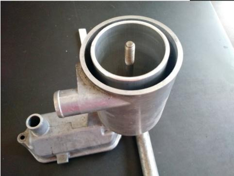
Place it into the oil separator as shown, then place the black cap back onto the oil separator and screw it down.
