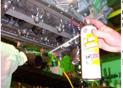
Each stud has a short end, a shoulder, and a long end. The short ends goes into the engine. The nut goes on the long end.
