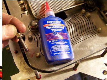
Install a stud in every hole EXCEPT the one immediately in front of the starter.
