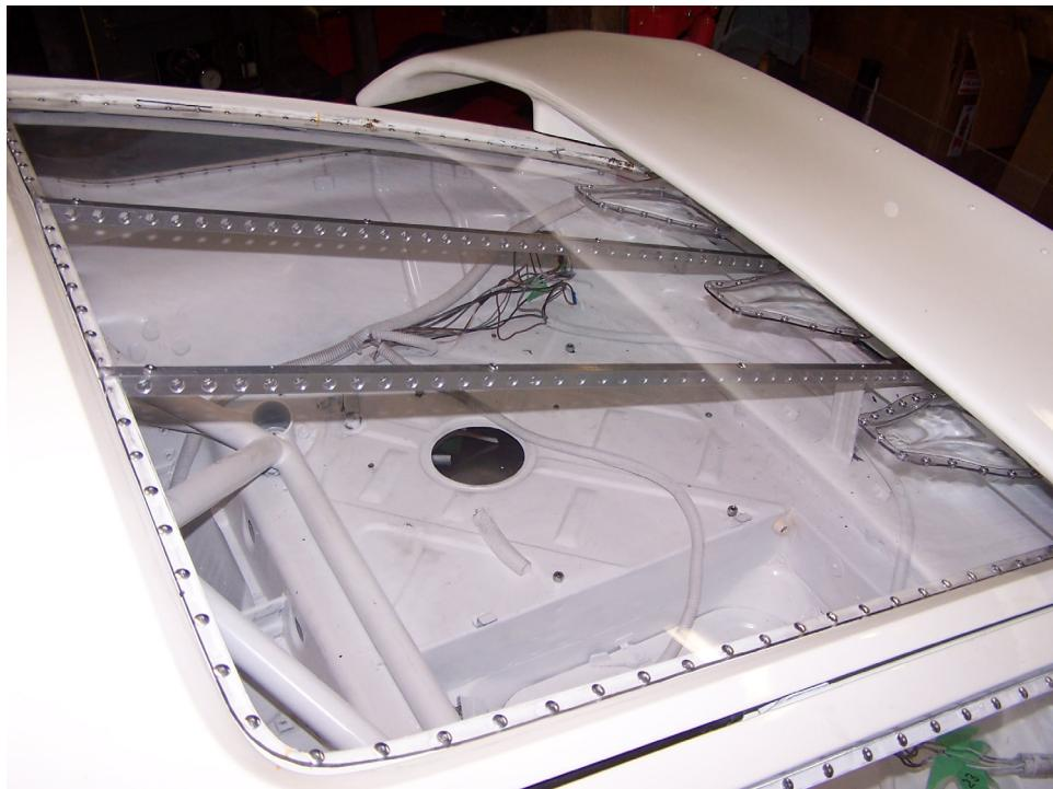
You MUST make some sort of brace or support for the large hatch window. I have seen a number of designs, and any one that works will do.
